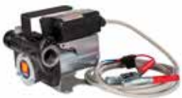
Art. 091-5081-060 12V Pump - power cable (sec. 4 mmq, 4 m lenght) with pincers and fuse - 60 l/min
