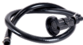
Art. 099-6510-011 Suction kit PU spiral hose 1,10 m length with SEC connection PVC spiral hose Ø 19x27 Inlet-outlet M 1" BSP SEC valve connection
